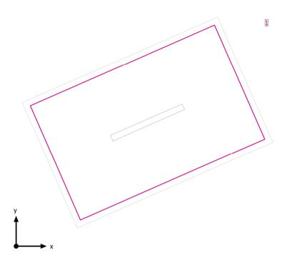
Clearance height: 2.800 m, Reflection factors: Ceiling 70.0%, Walls 50.0%, Floor 20.0%, Maintenance factor: 0.80
