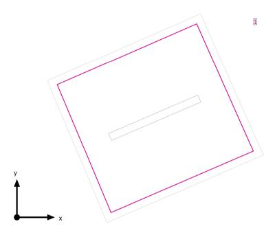
Clearance height: 2.800 m, Reflection factors: Ceiling 70.0%, Walls 50.0%, Floor 20.0%, Maintenance factor: 0.80
