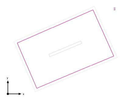
Clearance height: 2.800 m, Reflection factors: Ceiling 70.0%, Walls 50.0%, Floor 20.0%, Maintenance factor: 0.80
