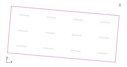
Clearance height: 3.000 m, Reflection factors: Ceiling 70.0%, Walls 50.0%, Floor 20.0%, Maintenance factor: 0.80
